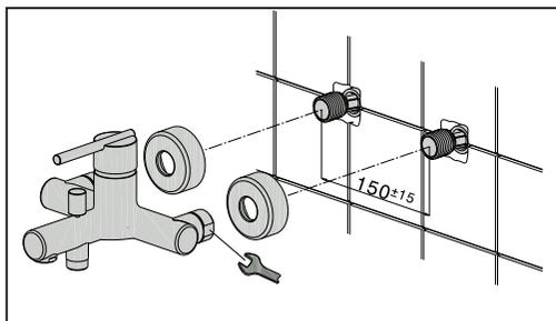
**SOSTITUZIONE DELLA VALVOLA MISCELATRICE A DISCHI CERAMICI**
