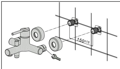
**SOSTITUZIONE DELLA VALVOLA MISCELATRICE A DISCHI CERAMICI**
